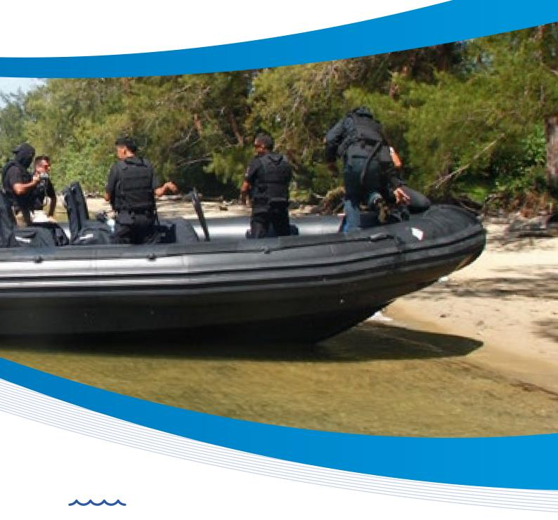
The RIB 9.5 Anti-Piracy vessel is specifically designed for long-duration, high-speed missions and equipped for Armed, Vessel Boarding Search & Seizure (VBSS)/ "Takedowns" critical to effective Anti-Piracy operations. Many options are available to include deck mounting of crew-serve weapons systems, tactical boarding ladders, FLIR Cameras and recording and wireless headset communication systems.
